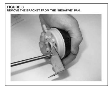
B. Replace the bracket to the "positive" pan as shown in Figure 4. The positive pan is the black colored half of the pressure switch that has the electrical terminals. Be careful to line up the alignment holes on the bracket with the nipples on the positive pan (see photo).
